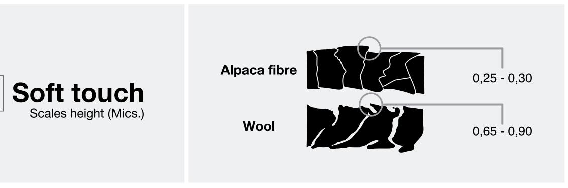
The finished yarn goes through two different processes. First, a bath is applied with water containing between 0.5% and 1% of UNIZIM PWO, an enzyme that eliminates chemically the scales found in each hair of the fiber, by eliminating the scales, felting is prevented.
